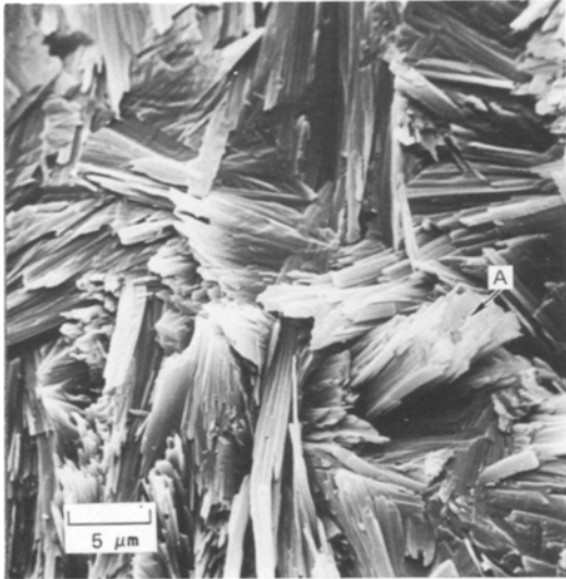
Figure 9 SEM showing cylindrical bundles of nephrite fibres, e.g. at A, in Russian jade.
